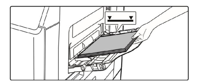
Insert the paper along the Bypass Tray Guides until it stops.
