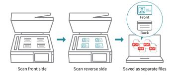
**Easy Scanning** Tap on the LCD touchscreen's Auto Set button to have the MFP perform a host of actions automatically. It can skip blank pages in a multi-page document or reorient pages mixed in upside down\*. The MFP also uses AI and image processing technology to automatically determine the optimal resolution, gradation, and compression rate for your scan jobs.
