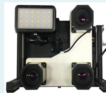
Triplet-lens camera rebar arrangement inspection system
