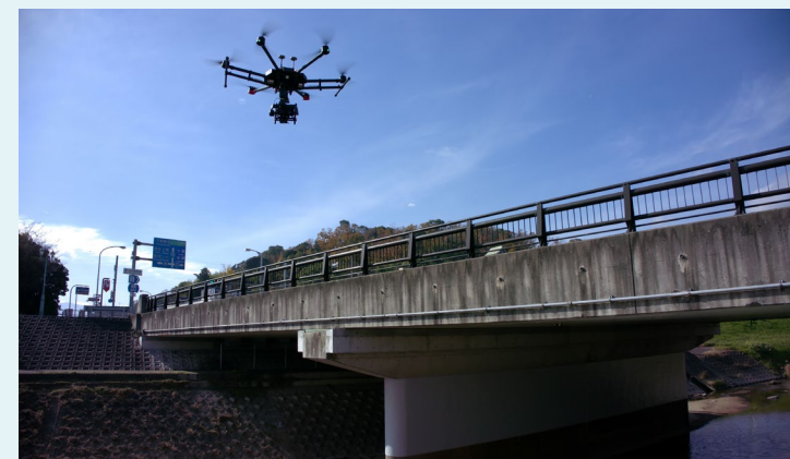
8K-camera drone on an aerial inspection
