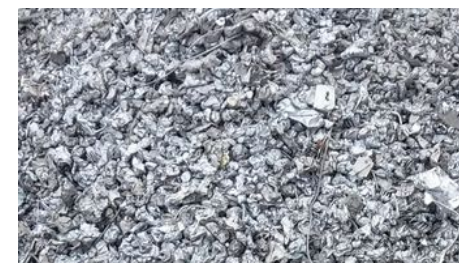
Iron recovered by magnetic separator
